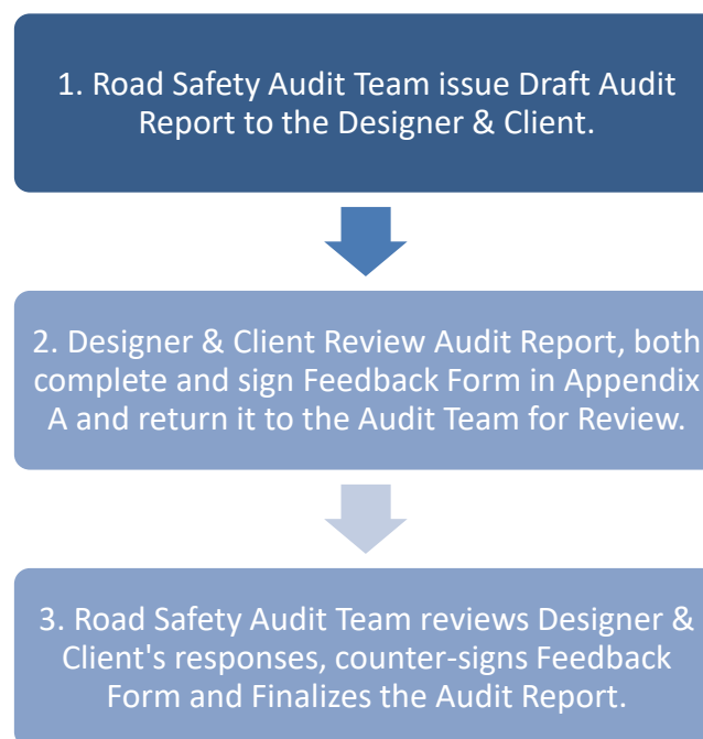
Figure 4.1 – Road Safety Audit Sign-Off and Completion Process
